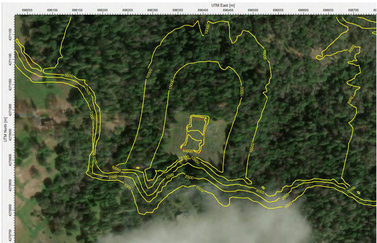
Figure 3 Contours of Relative Odor Concentration (in micrograms per cubic meter)
