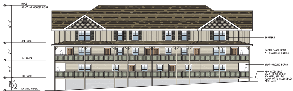
2 EXTERIOR ELEVATION - BUILDING B SOUTH (FRONT)
