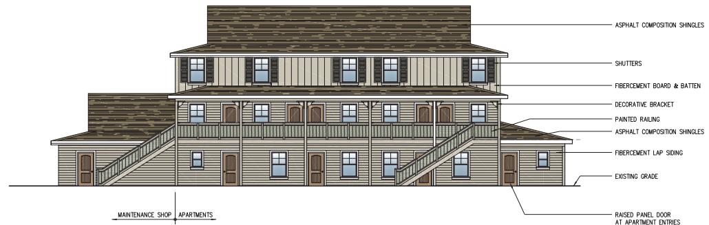
3 EXTERIOR ELEVATION - BUILDING C SOUTH (FRONT)
