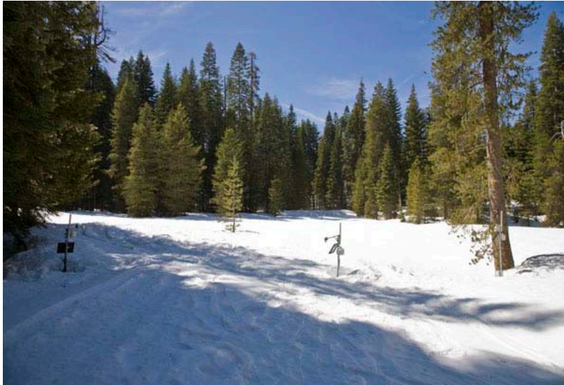
Photo 4. Snow-depth sensors in Southern Sierra CZO meadow and adjacent forest.
