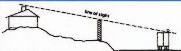
4.16 To be effective, a barrier must block the "line of sight" between the highest point of a noise source and the highest part of a receiver.
