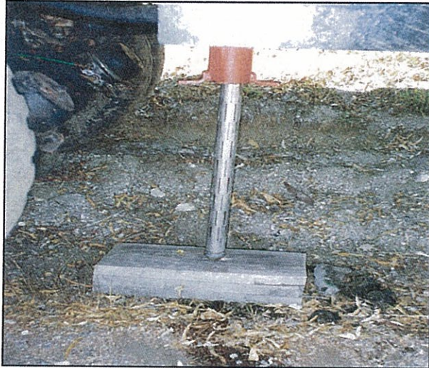
FIGURE 5 OILFIELD MILL SLOT SCREEN
