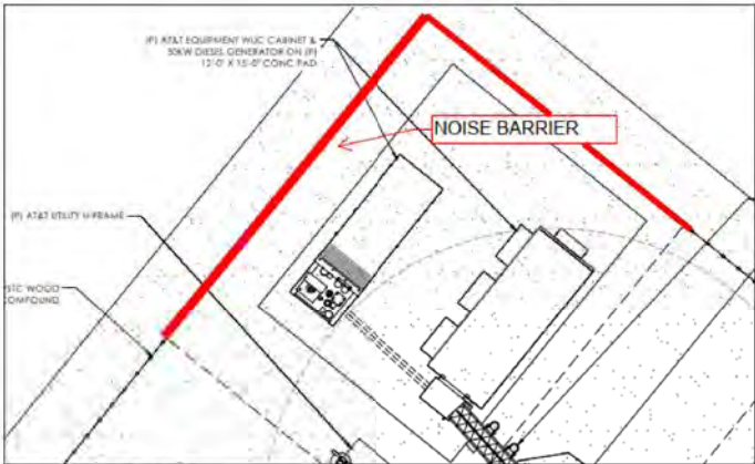
Figure 2: Noise Barrier - Plan
