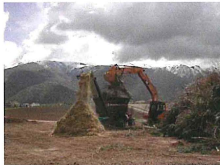
Grinding green waste
