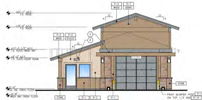
2 RIGHT ELEVATION- EAST SIDE SCALE: 3/16"=1'-0"
