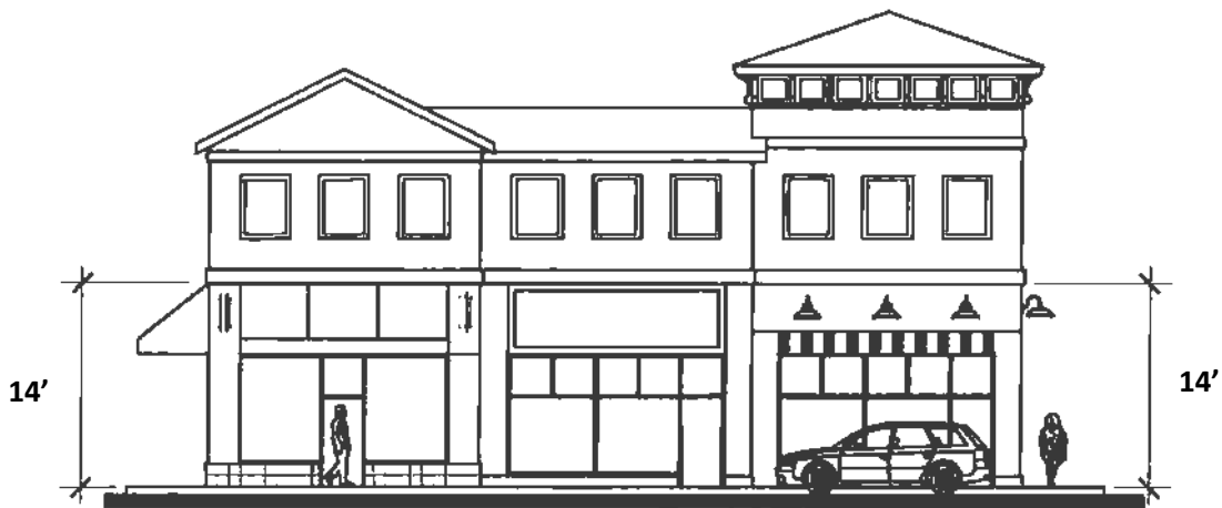
Figure 4.3-1. MIXED USE GROUND FLOOR HEIGHT
