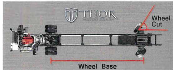
Diesel Motorhome Chassis: The Wheel Cut & Wheel Base Effect On Turning Radius
