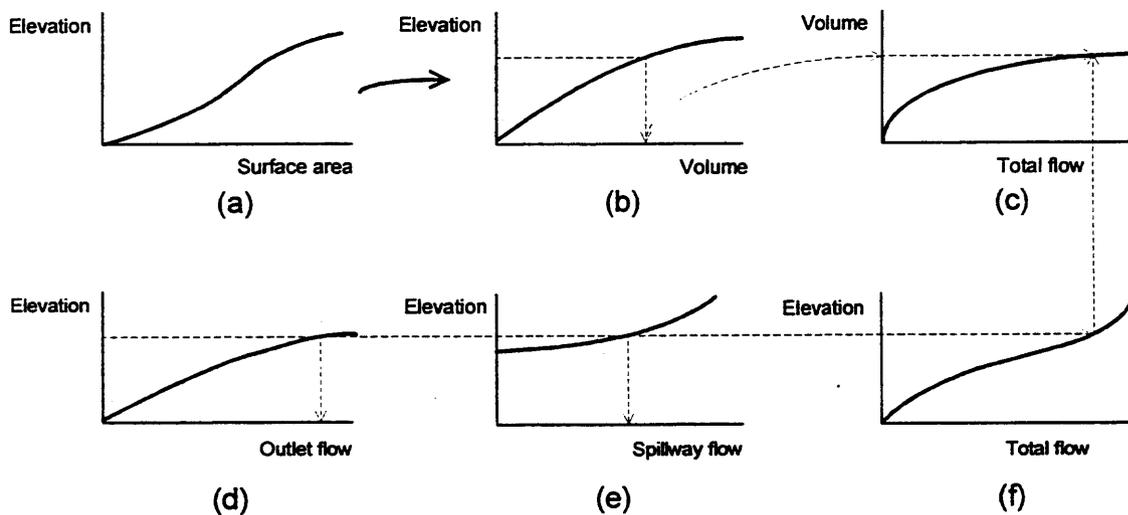
**FIG. 5.7.1 Derivation of Storage-outflow Relationship**
