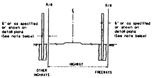
NOTE: Offset to be 2'-0" at monument locations, measured at right angles to R/R lines. Taper to achieve offset to be at least 20' long.
