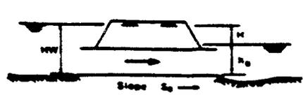
SUBMERGED OUTLET CULVERT FLOWING FULL
