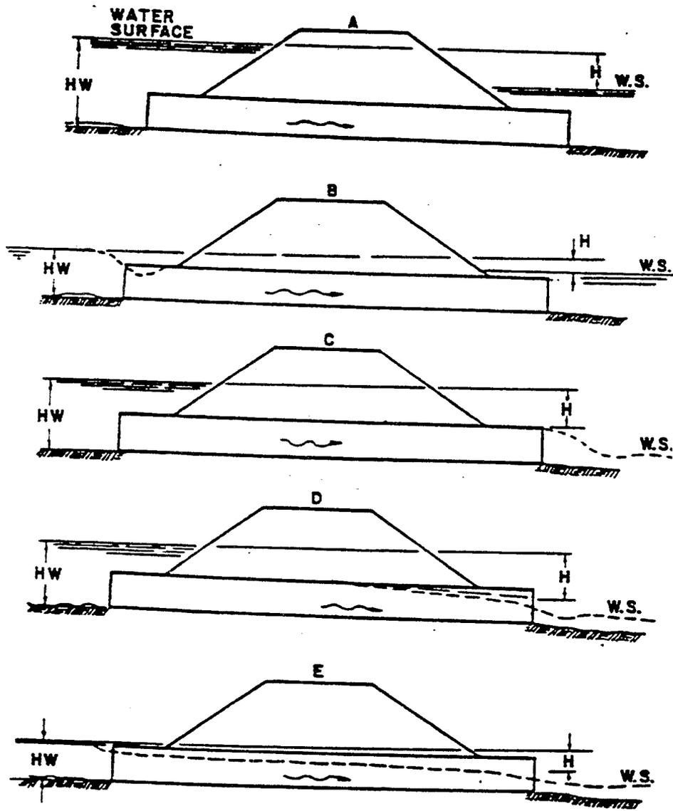
Figure 7.2.2 Schematic Diagram Showing Types of Outlet Control for Culvert Flow.
