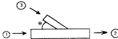
Figure 4.2.1 Schematic Diagram of Pipe Junction.
