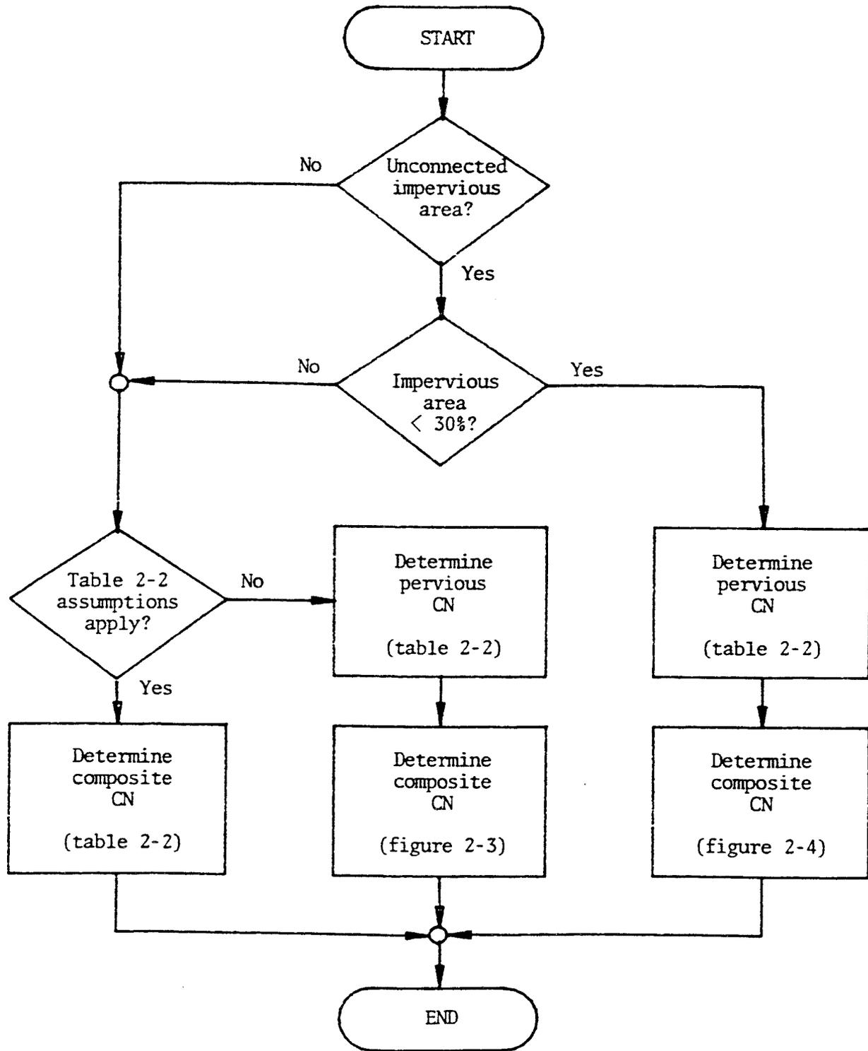
Figure 2-2.—Flow chart for selecting the appropriate figure or table for determining runoff curve numbers.
