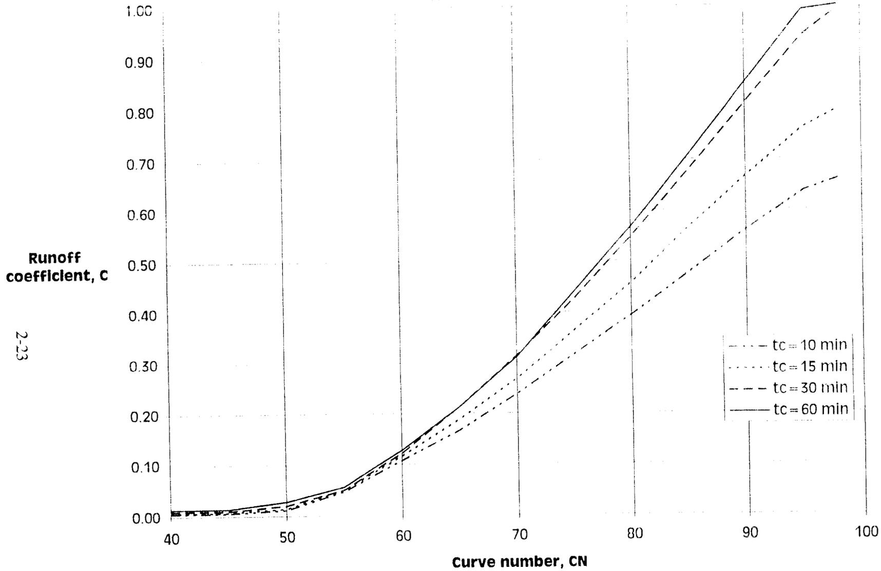
**Fig. 2.5.4 Runoff Coefficients for 100-yr Event below 1,640'**
