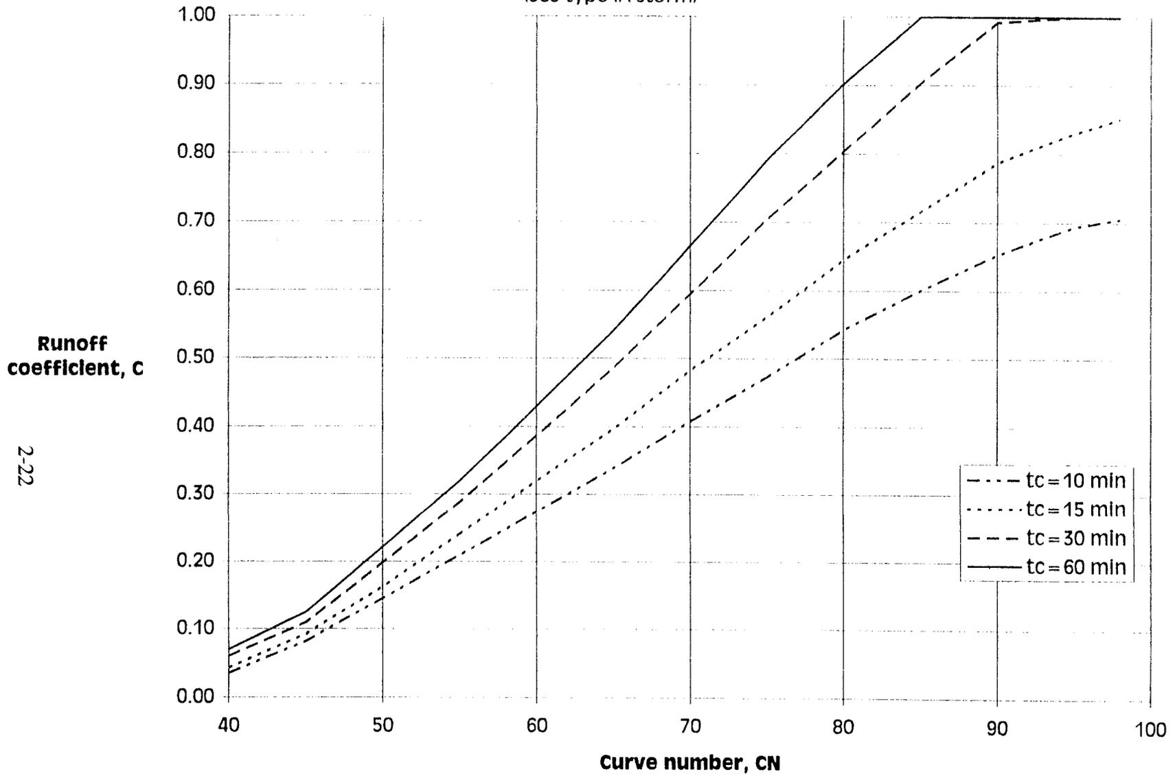
**Fig. 2.5.3 Runoff Coefficients for 10-yr Event below 1,640'**
