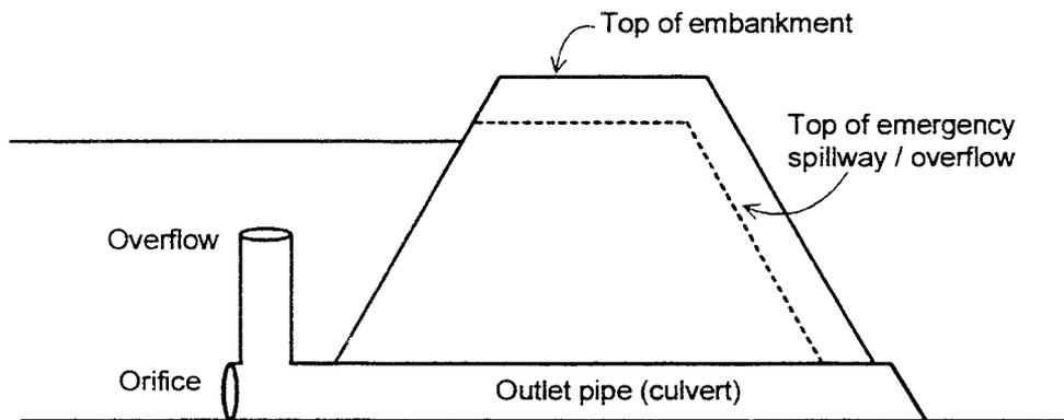
**Fig. 5.2.2 Typical Detention Structure**
