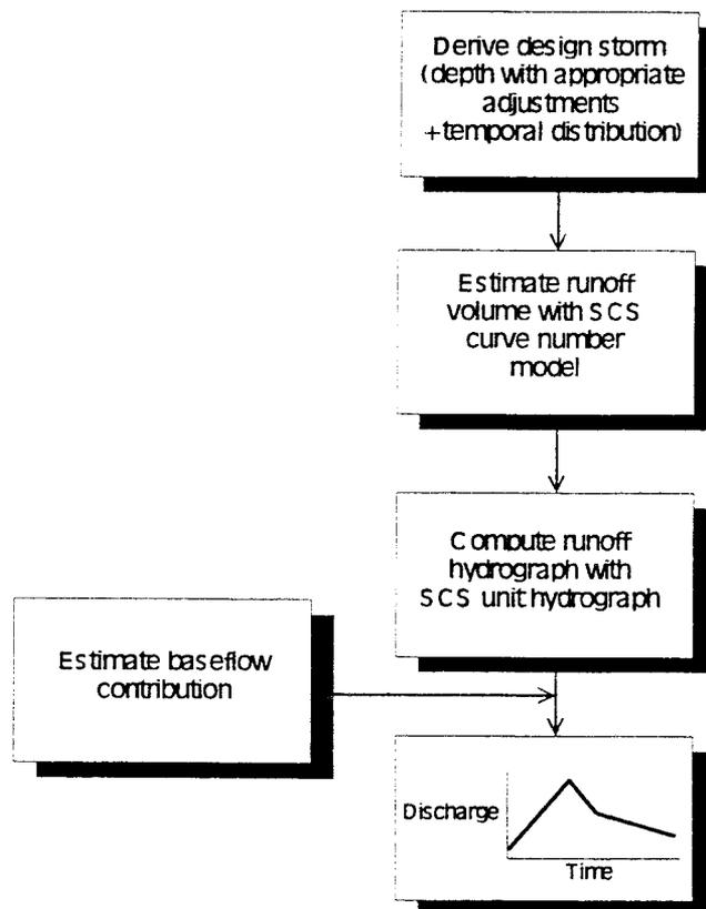
FIG. 2.4.1 Runoff Computation Procedure
