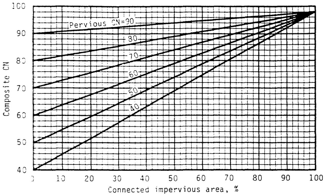
Figure 2-3.—Composite CN with connected impervious area.
