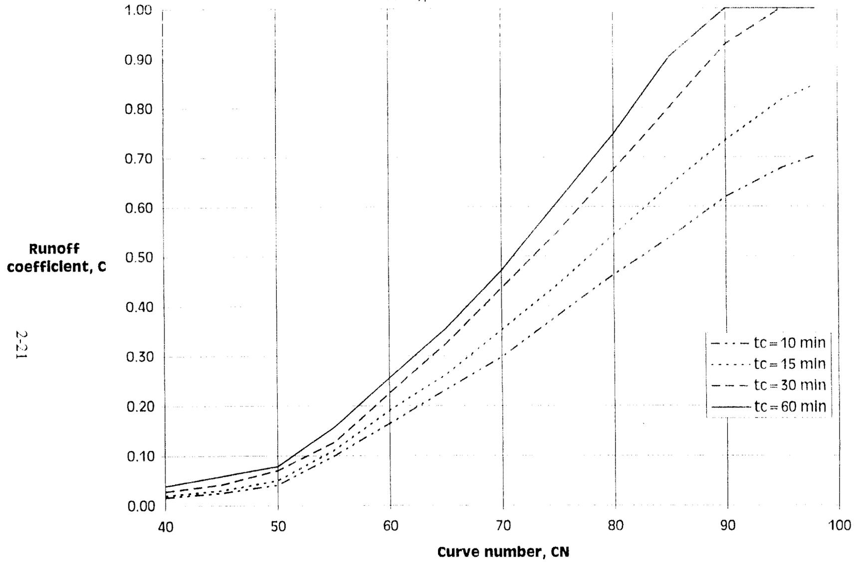
**Fig. 2.5.2 Runoff Coefficients for 100-yr Event above 1,640'**
