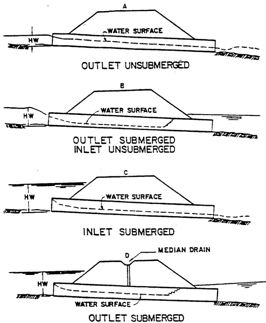
Figure 7.2.1 Schematic Diagram of Types of Inlet Control for Culvert Flow.
