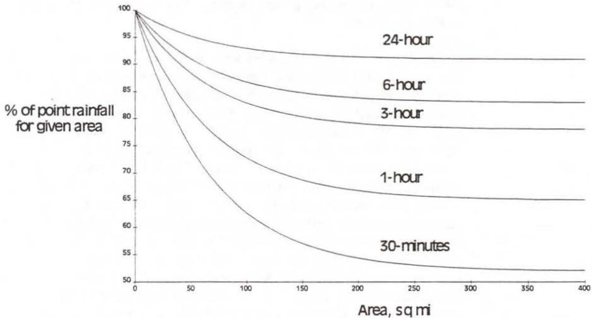
**FIG. 2.3.1 Depth-area Adjustment**
