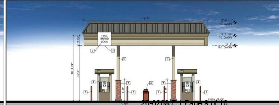
4 FUEL CANOPY ELEVATION: REAR (NORTH)
