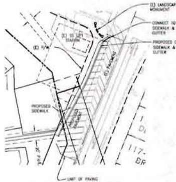
SIDEWALK/BIKE PATH CONNECTION DETAIL SCALE: 1"=40'
