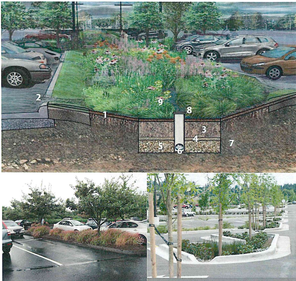
Figure 32. Examples of parking lot planters and rain gardens
