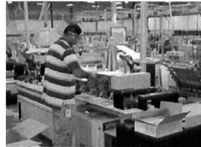
A technician moves printed statements through an advanced envelope insertion machine.
