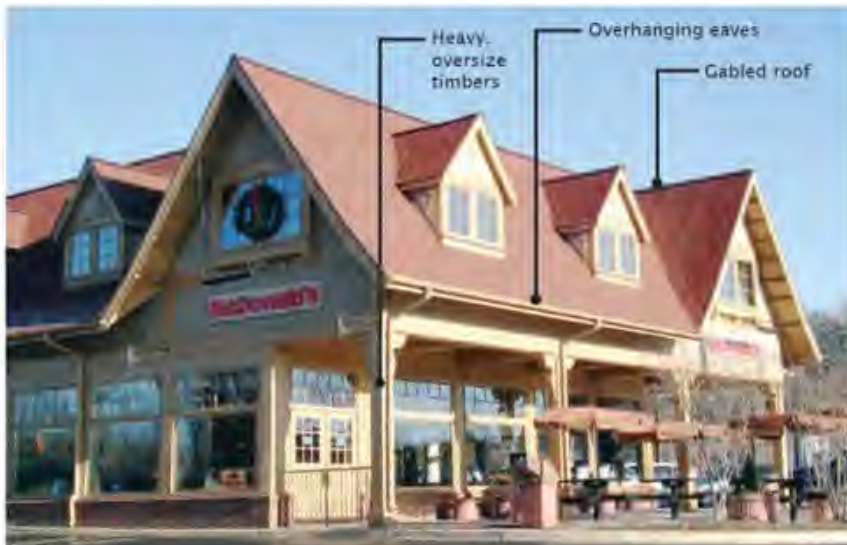
Figure 2. Typical Design Features of the Mountain/Lodge Style
