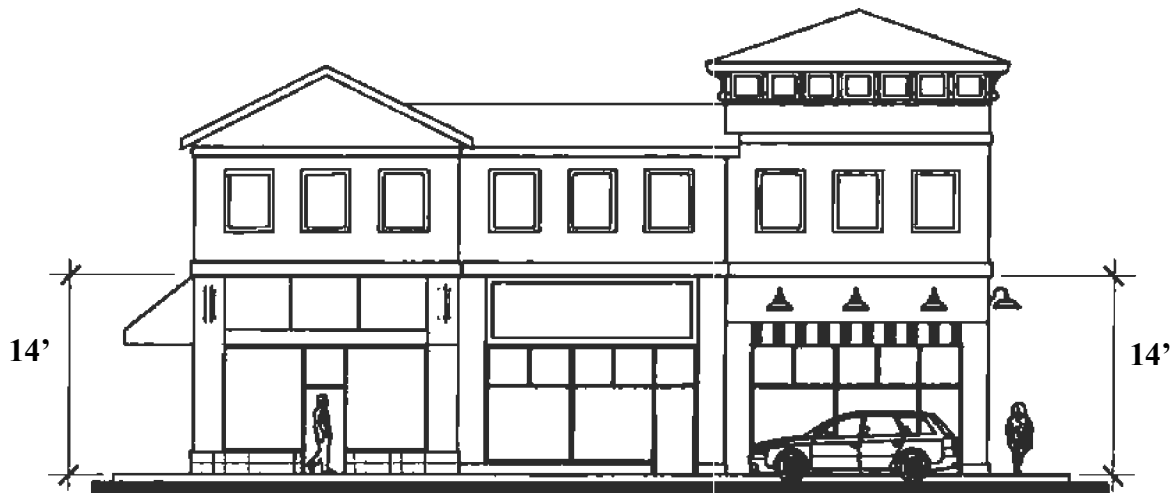
FIGURE 3.1-1. MIXED USE GROUND FLOOR HEIGHT
