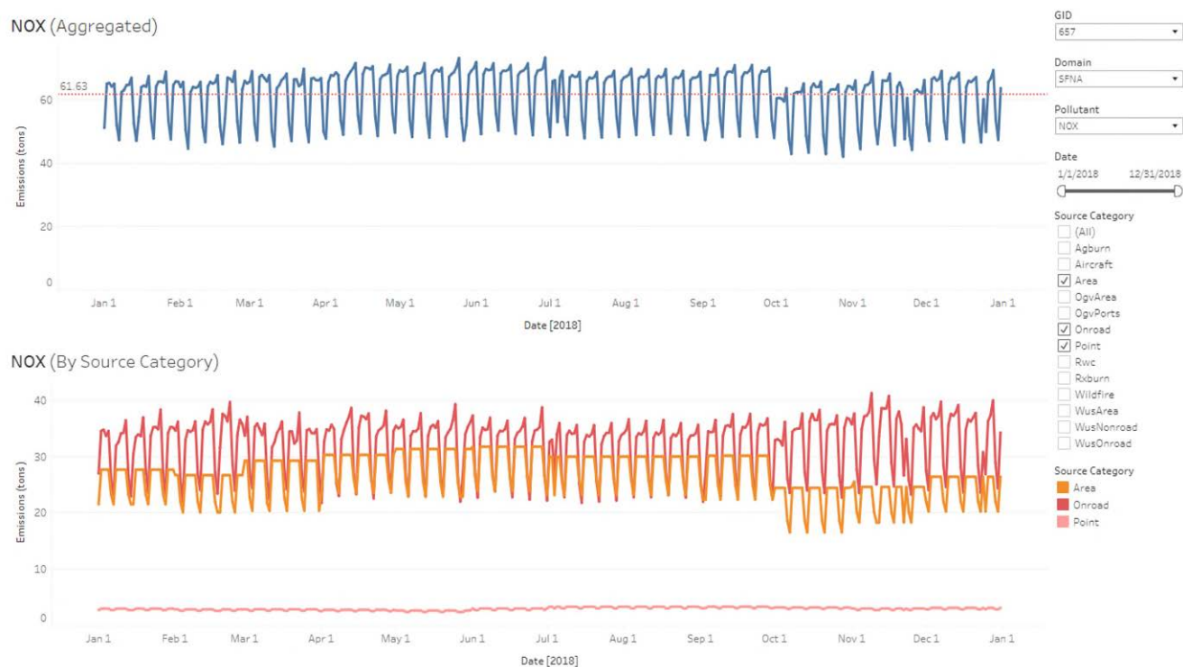
Figure B-30: Example timeseries plot for daily 2018 NO x emissions from area, on-road, and point sources for Sacramento Nonattainment Area
