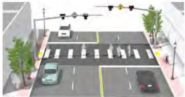
Figure 6-11: Example of a Pedestrian Hybrid Beacon
