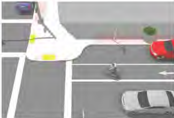
Figure 6-8: Example of a curb extension
