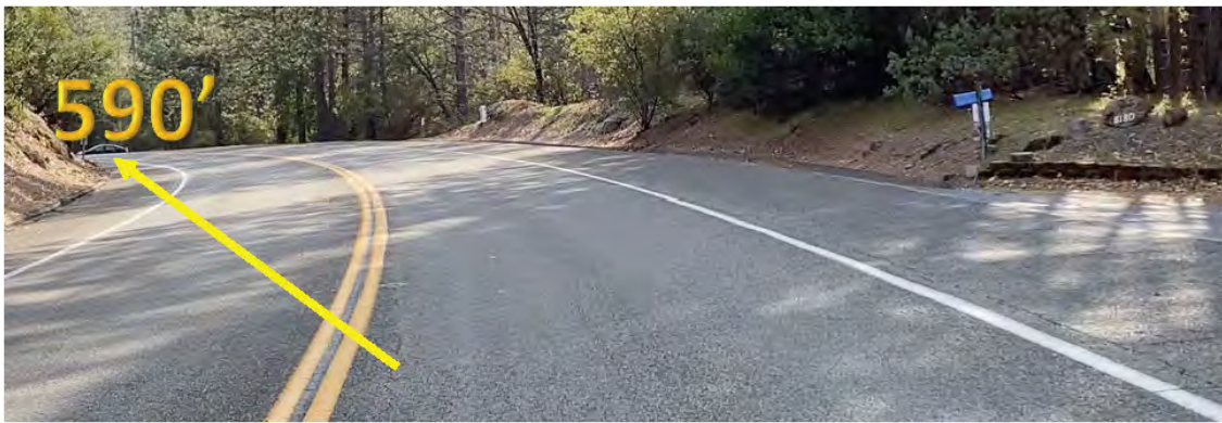
FIGURE 7. SIGHT DISTANCE, MT AUKUM RD SOUTHBOUND AND NORTHBOUND
