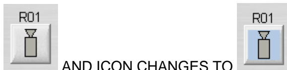
Select any CAMERA pushbutton icon to view the image the video surveillance system monitor. The CAMERA icon pushbutton is BLUE while the camera is active. Select another camera to change the active video image.
