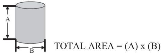
Figure 130.36.070.D Area of Three-Dimensional Objects
