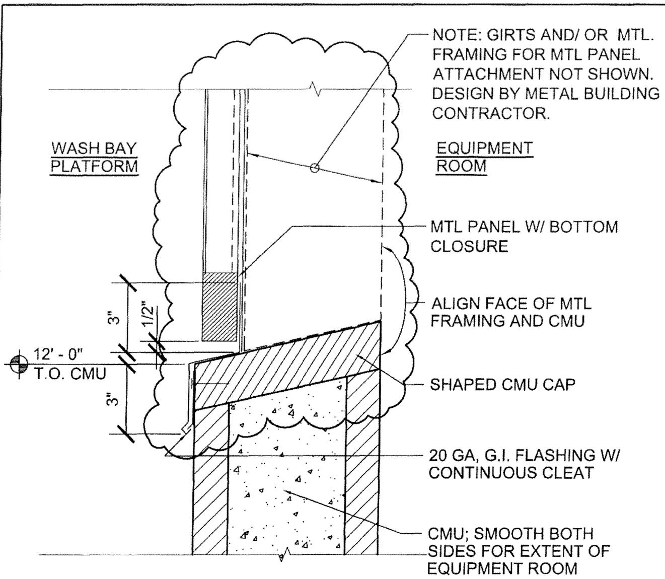
**3 FLASHING DETAIL @ CMU WALL**
