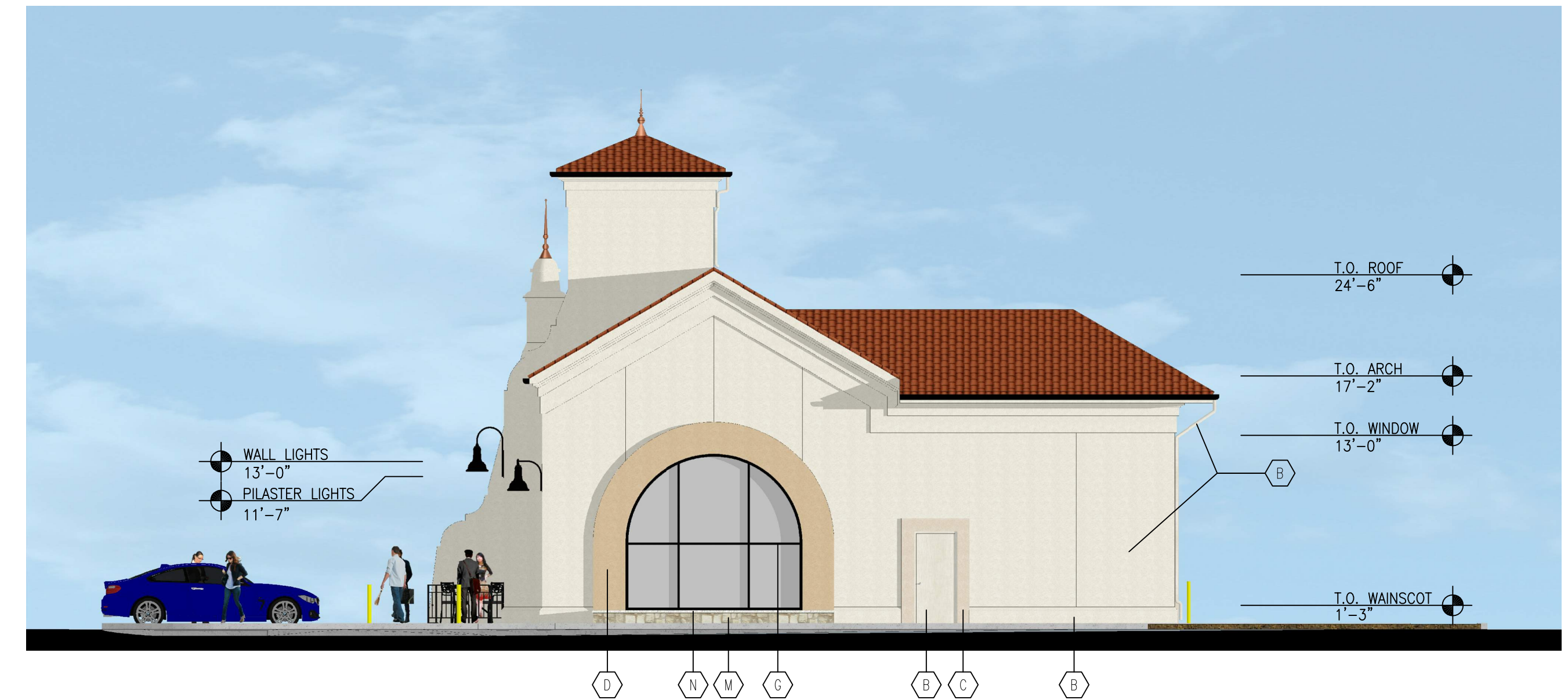
BUILDING 2A - NORTH ELEVATION
