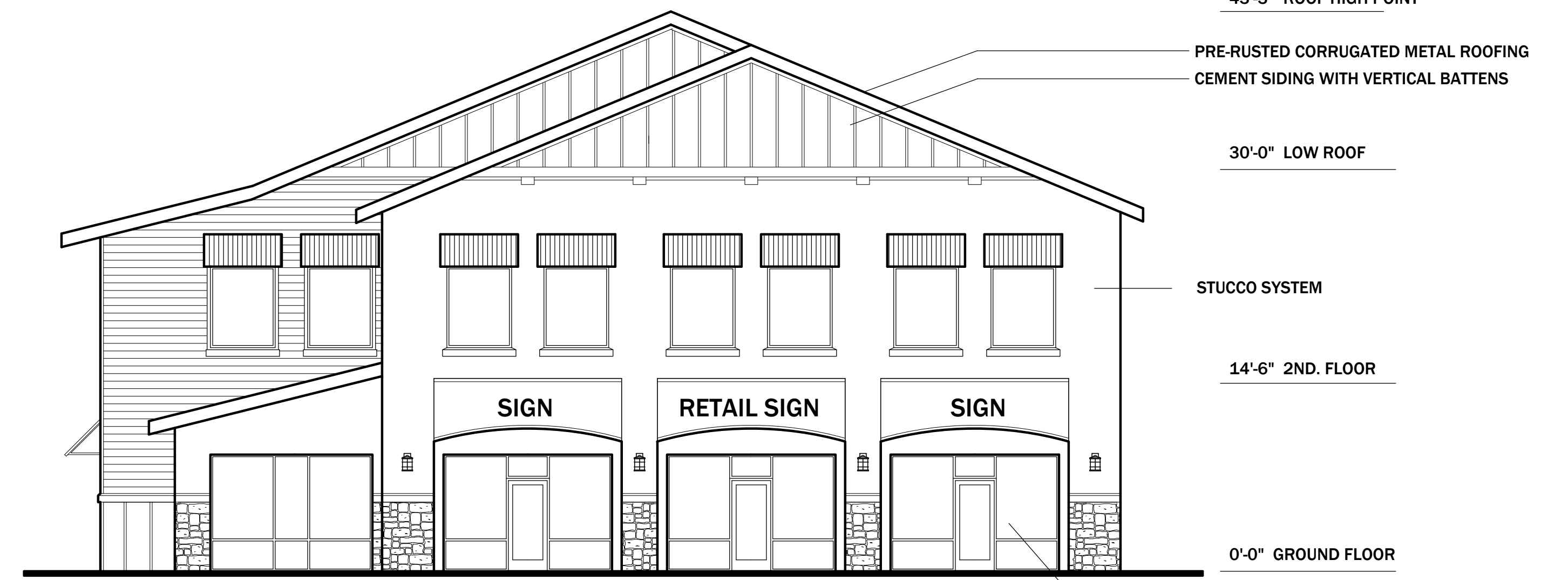
ELEVATION FROM M. FLAT ENTRY DRIVE ( SOUTH)
