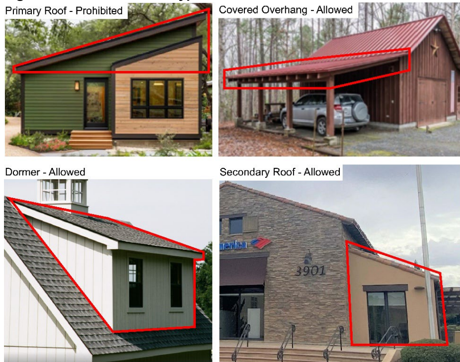
Figure 7 Shed Roof Types
