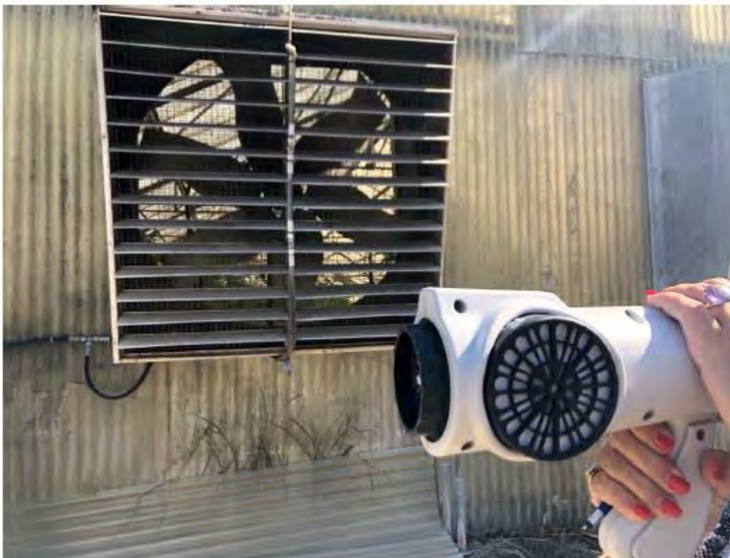
Figure 11 Field Measurements of Odor Intensity Using Nasal Ranger Oct 1-3, 2019
