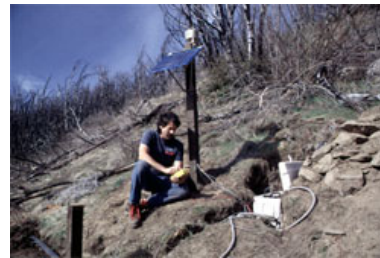
Photo 4: Testing the solar-powered radio telemetry system used for real-time monitoring. USGS Photo by Mark Reid, USGS/Menlo Park
