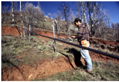
Photo 5: Measuring landslide movement using a surface extensometer. Extensometer crosses several scarps (breaks that expose the reddish soils) at the head of the landslide. USGS Photo by Richard LaHusen, USGS/CVO
