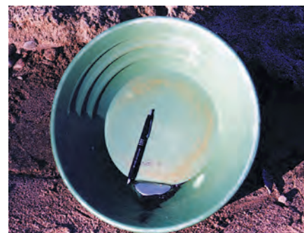
Figure 3. Gold pan with more than 30 grams of mercury from 1 kilogram of mercury-contaminated sediments collected in a drainage tunnel.
