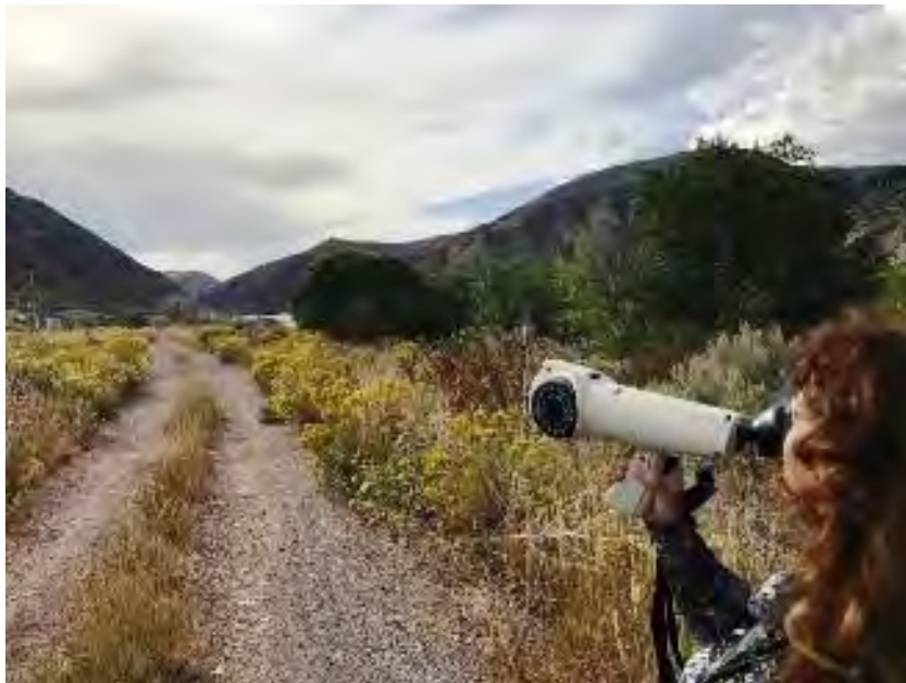
Figure No. 1 – Nasal Ranger Olfactometer
