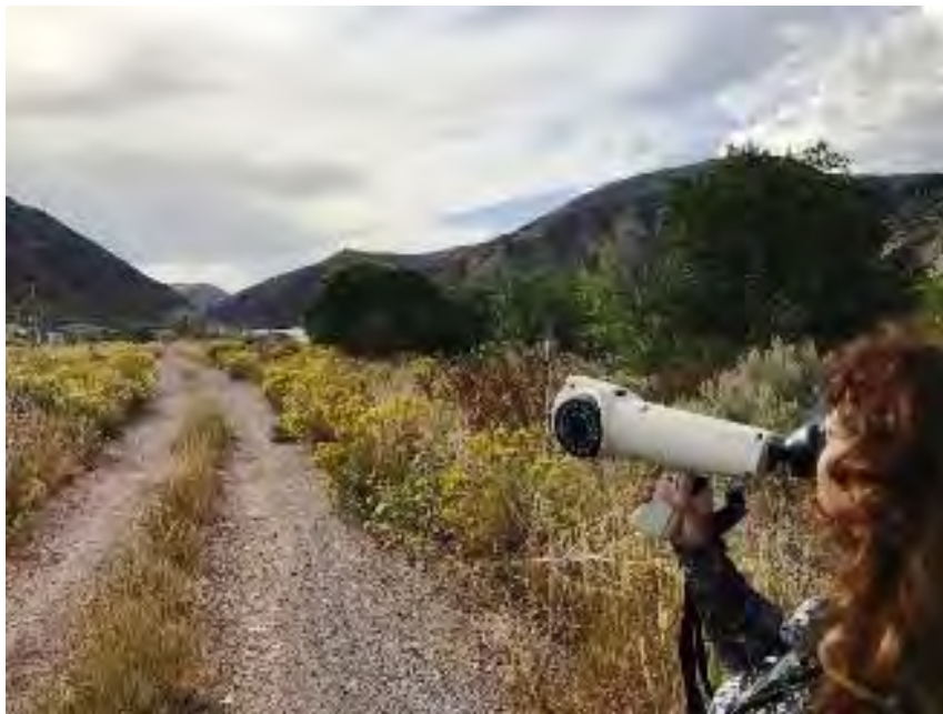
Figure No. 1 – Nasal Ranger Olfactometer
