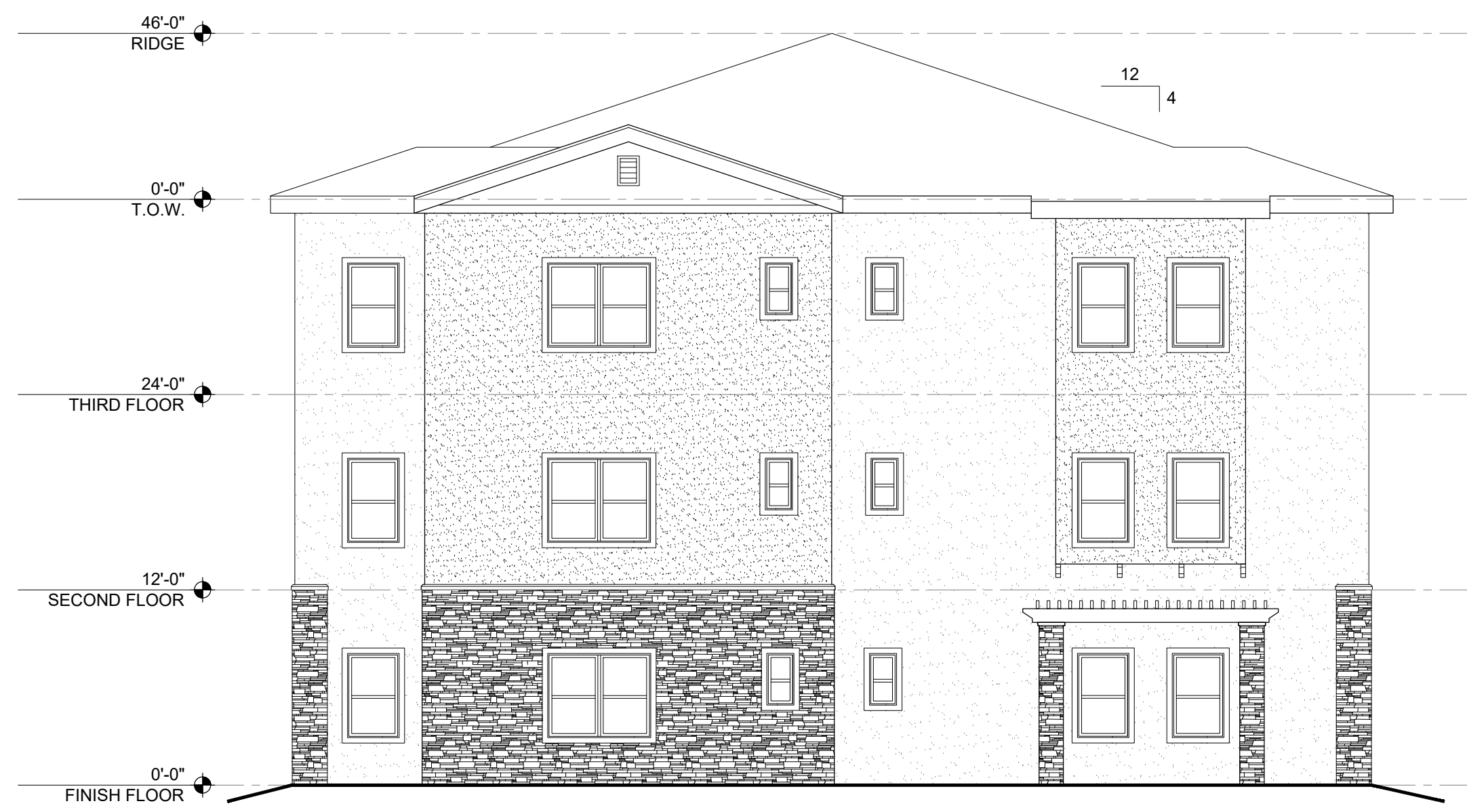
2 EXTERIOR ELEVATION - TYPE B 1/8" = 1'-0"
