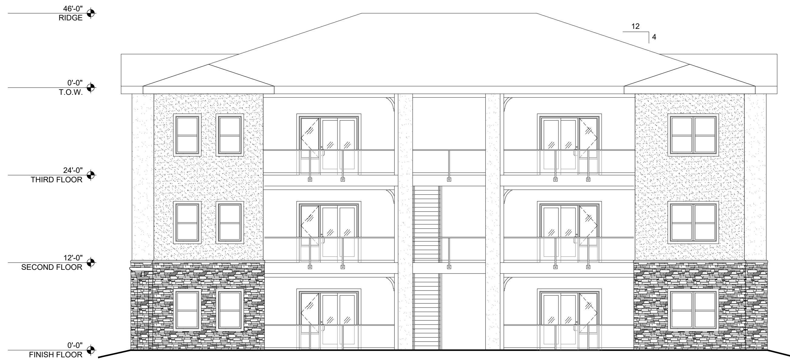
4 EXTERIOR ELEVATION - TYPE B 1/8" = 1'-0"
