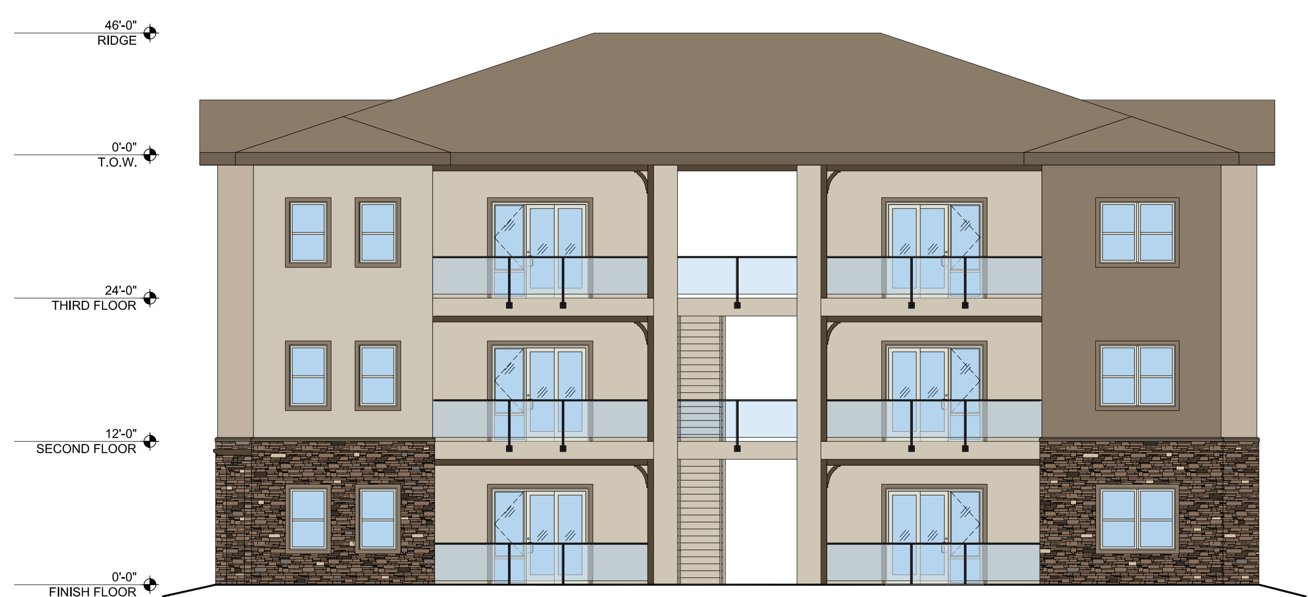
4 EXTERIOR ELEVATION - TYPE B 1/8" = 1'-0"
