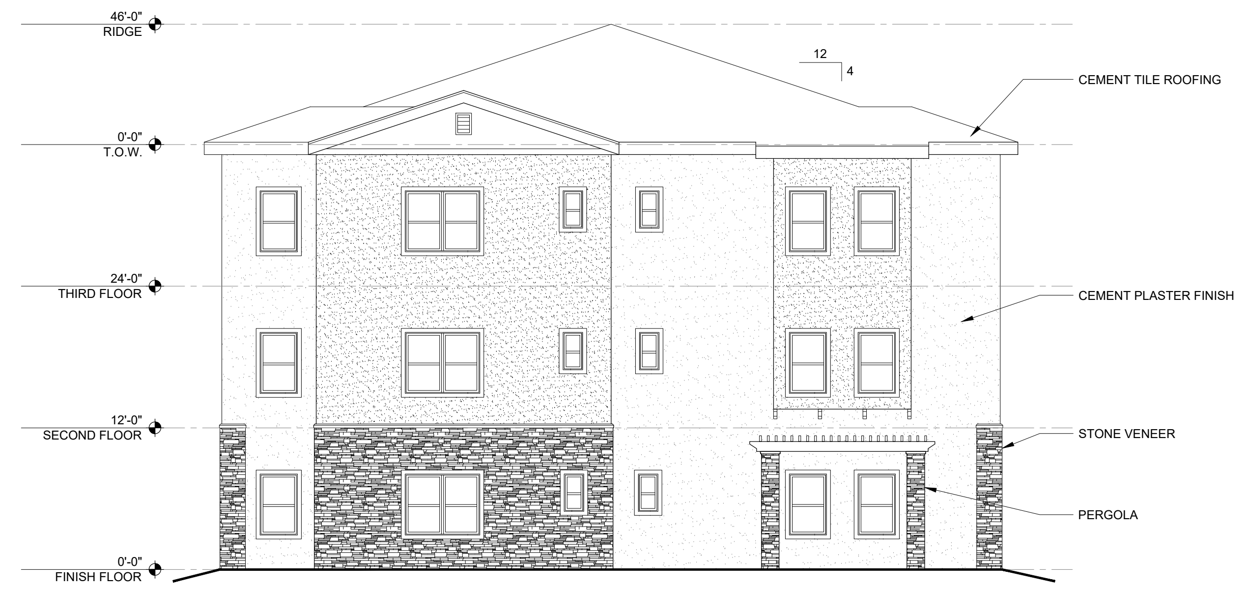
3 EXTERIOR ELEVATION - TYPE B 1/8" = 1'-0"
