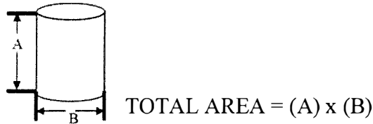
Figure 130.36.070.D Area of Three-Dimensional Objects
