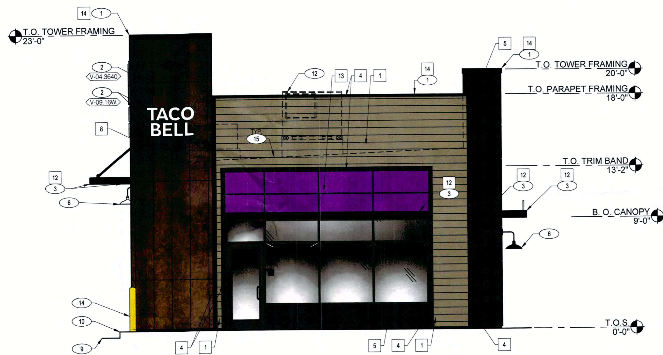
SOUTH ELEVATION 1/4" = 1'-0" C
