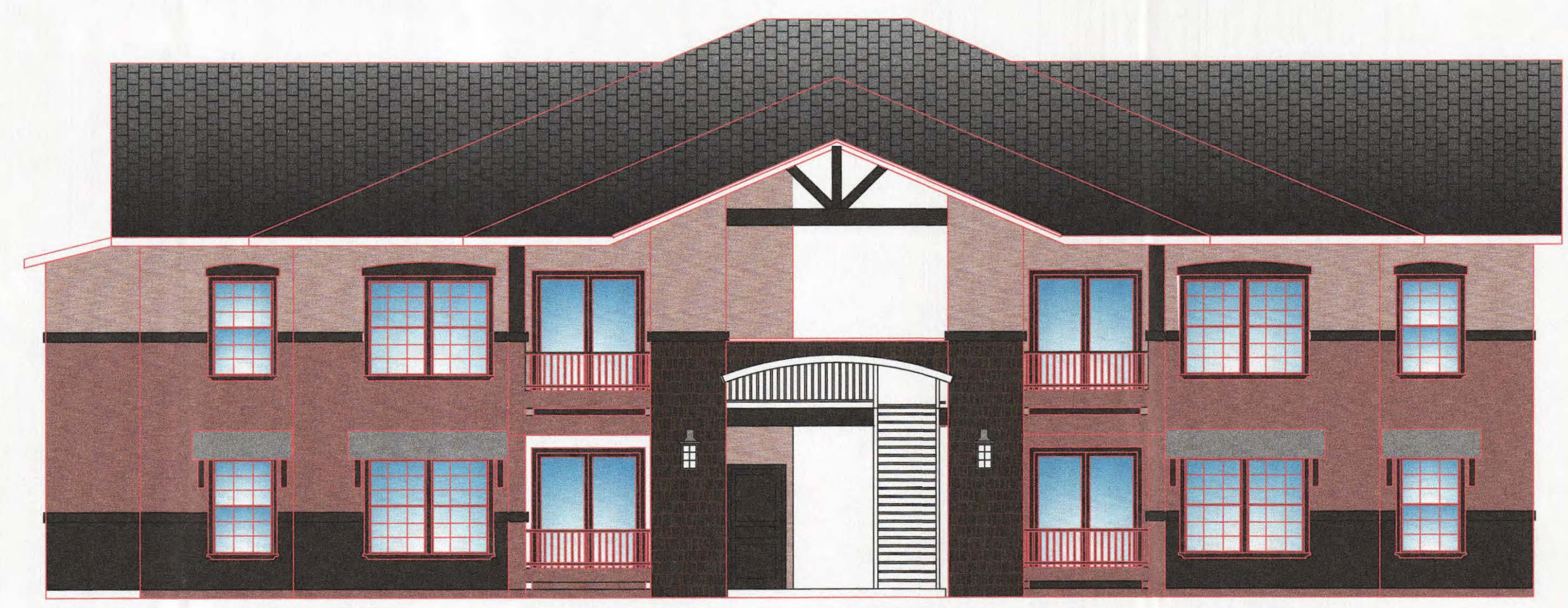
2-BDRM ELEVATION 1 FRONT / REAR 1/6"=1'-0"
