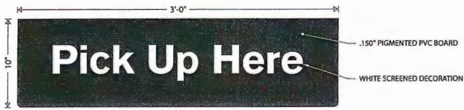
WINDOW POSITION SIGN DETAILS SCALE: 1 1/2" = 1'-0"
