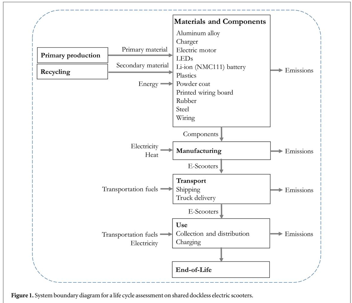
Figure 1. System boundary diagram for a life cycle assessment on shared dockless electric scooters.
