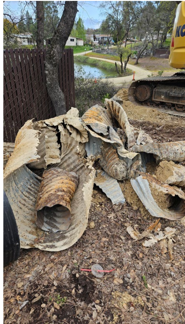
Damaged/destroyed culvert removed from roadway
