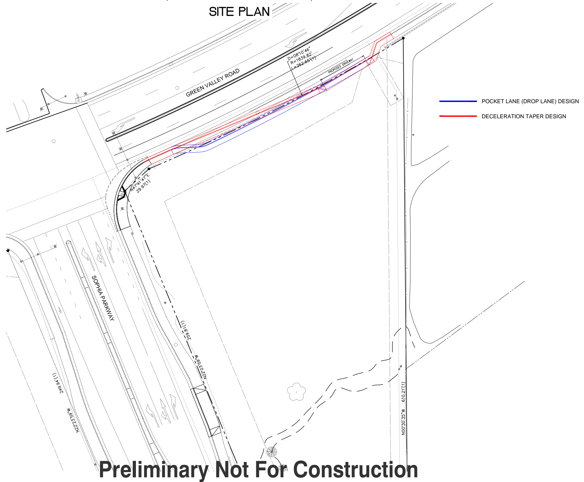
Figure 3.0-1 Deceleration Taper and Drop Lane Comparison
