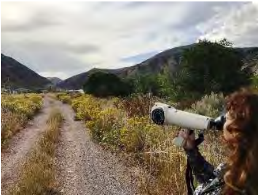
Figure No. 1 – Nasal Ranger Olfactometer
