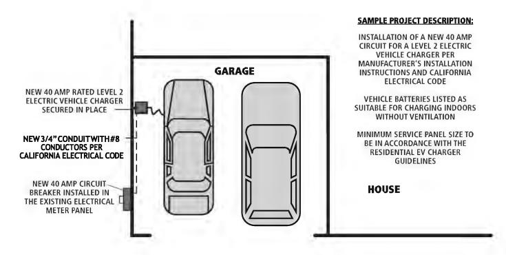
Though an individual Level 2 EV charger may have a negligible impact on the utility electric system, the combined effect of several chargers in the same neighborhood could result in overloads on utility secondary wires and transformers. It is important that the local SCE office (SCE Planning 805-654-7444) be notified of any Level 2 charger installations to ensure that utility electrical system components are adequately sized to maintain high levels of service reliability.
