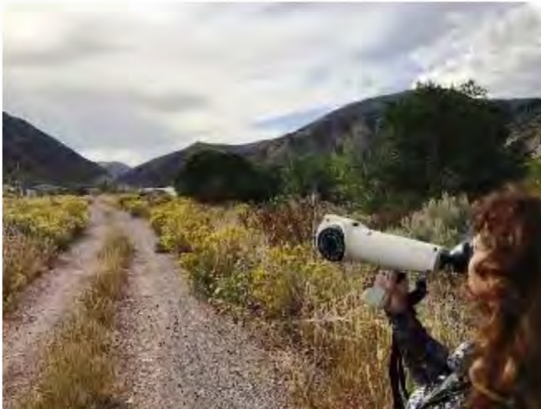
Figure No. 1 – Nasal Ranger Olfactometer
