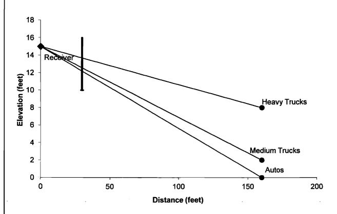
Centerline to Barrier Distance (C<sub>1</sub>): 130 Barrier to Receiver Distance (C2): 30 0 Automobile Elevation: 2 Medium Truck Elevation: **Heavy Truck Elevation:** 8 Pad/Ground Elevation at Receiver: 10 Receiver Elevation<sup>1</sup>: 15 10 Base of Barrier Elevation: Barrier Height<sup>2</sup>:
