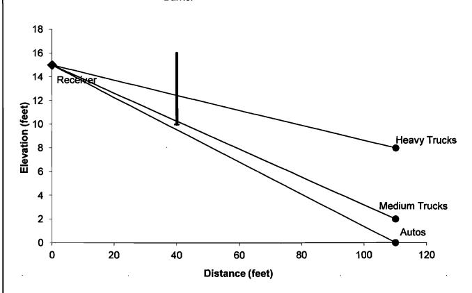
Centerline to Barrier Distance (C<sub>1</sub>): 70 Barrier to Receiver Distance (C2): 40 Automobile Elevation: 0 2 Medium Truck Elevation: **Heavy Truck Elevation:** 8 Pad/Ground Elevation at Receiver: 10 Receiver Elevation 1: 15 Base of Barrier Elevation: 10 Barrier Height<sup>2</sup>:
