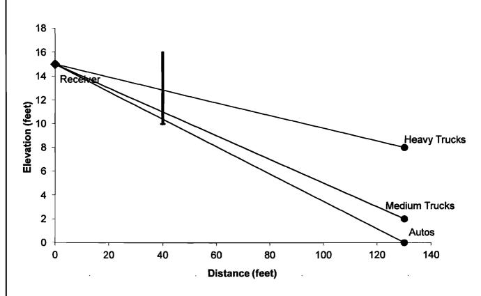
Centerline to Barrier Distance (C<sub>1</sub>): 90 Barrier to Receiver Distance (C2): 40 Automobile Elevation: 0 2 **Medium Truck Elevation:** 8 **Heavy Truck Elevation:** Pad/Ground Elevation at Receiver: 10 Receiver Elevation 1: 15 Base of Barrier Elevation: 10 Barrier Height<sup>2</sup>: 6
