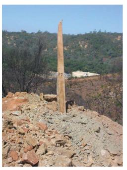
Figure 4-6. Rock not suitable for rock fill embankment: materials closer to soil than rock.
