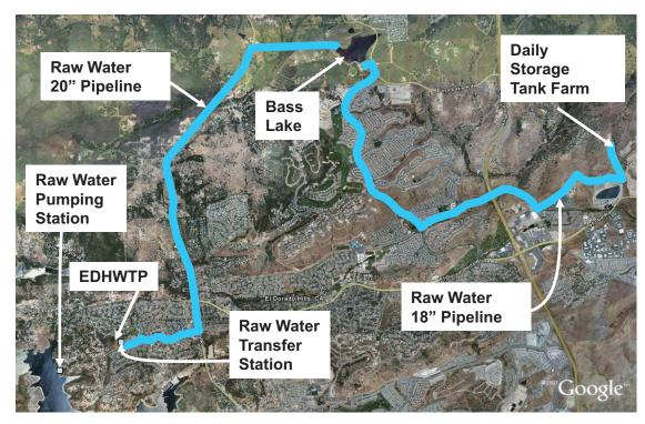
Figure 5-5. Raw Water Pumping and Pipeline to Bass Lake and Tank Farm, Alternative 3A
