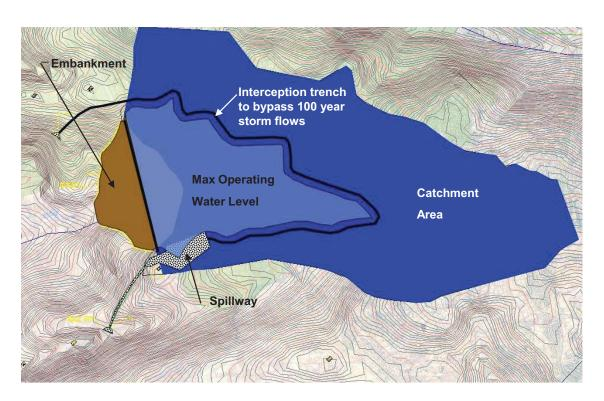
Figure 4-9. Deer Creek Embankment Alignment, Reservoir, and Catchment Area
