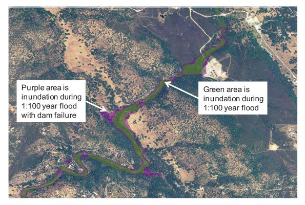
Figure 4-10. Inundation During Embankment Failure at Deer Creek Site During 1:100 Year Storm in Purple and 1:100 Year Flood Flow in Green
