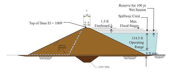
Figure 4-8. Section through the Embankment at the Deer Creek Reservoir
