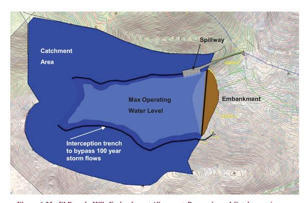
Figure 4-25. El Dorado Hills Embankment Alignment, Reservoir, and Catchment Area
