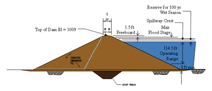
Figure ES-5. Typical Cross-Section of the Embankment for the El Dorado Hills Site
