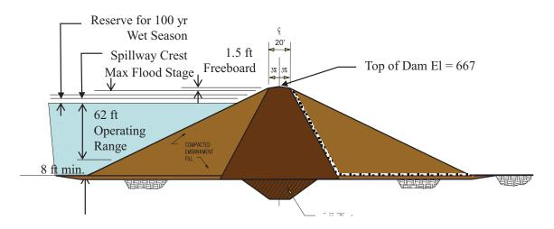
Figure 4-24. Section through the Embankment at the El Dorado Hills Reservoir
