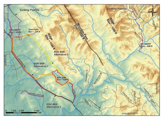
Figure 4-29. Pipeline Routes from the Reservoir Pumping Station to the Daily Storage Tank Farm with Seasonal Storage at the El Dorado Hills Reservoir Site
