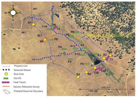
Figure 4-14. Final Plan for Geological Site Evaluation – El Dorado Hills Site
