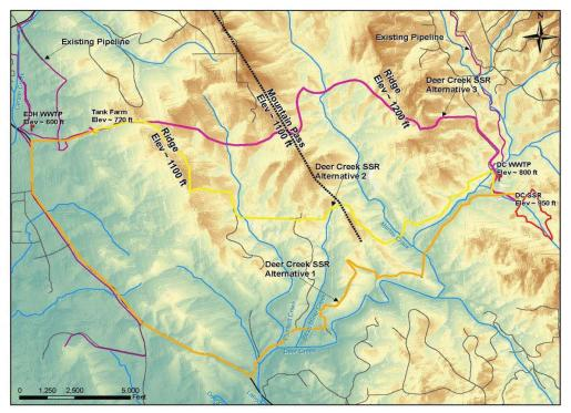
Figure 4-13. Pipeline Routes from the Reservoir Pumping Station to the Daily Storage Tank Farm with Seasonal Storage at the Deer Creek Reservoir Site
