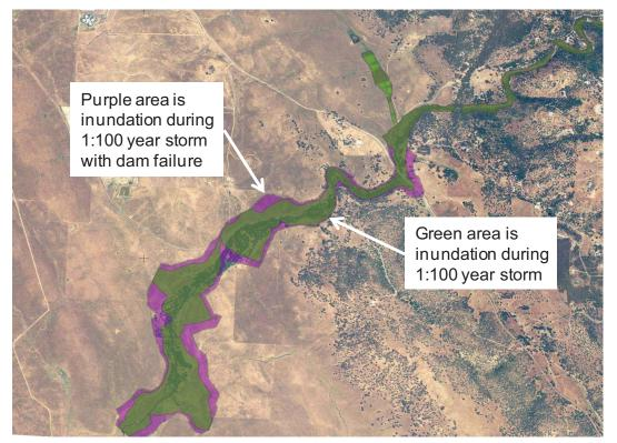
Figure 4-26. Inundation due to Embankment Failure at El Dorado Hills Site During 1:100 Year Storm in Purple and 1:100 Year Storm Event shown in Green.
