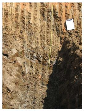
Figure 4-18. Bedrock Deeply Weathered and Sheared, Highly Fractured
