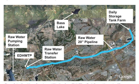
Figure 5-6. Raw Water Pumping and Pipeline from EDHWTP to Tank Farm, Alternative 2B
