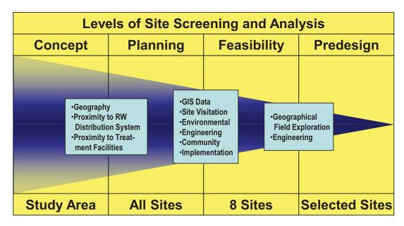
Figure 3-1 Screening Steps for Potential Recycled Water Seasonal Storage Reservoir Sites
