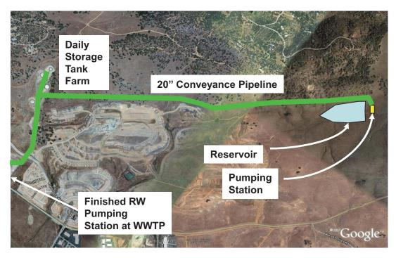
Figure 5-3. Recycled Water Seasonal Storage Reservoir, Pump Stations, and Piping, Alternative 2
