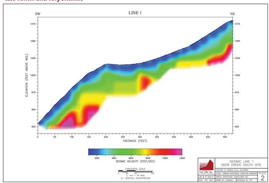
Figure 4-7. Seismic Refraction Survey Results – Deer Creek Site
