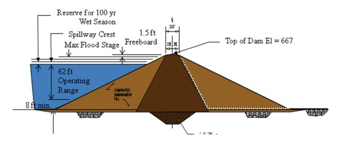
Figure ES-4. Typical Cross-Section of the Embankment for the Deer Creek
