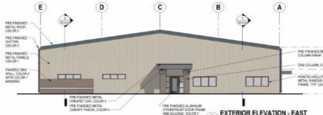
3 EXTERIOR ELEVATION - EAST
