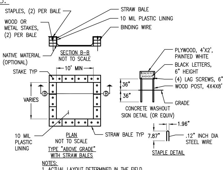
1. ACTUAL LAYOUT DETERMINED IN THE FIELD. 2. THE CONCRETE WASHOUT SIGN SHALL BE INSTALLED WITHIN 32' OF THE TEMPORARY CONCRETE WASHOUT FACILITY.
