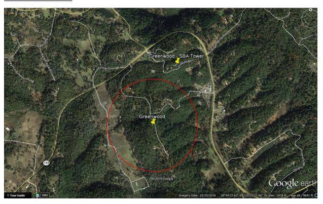
The nearby SBA Wireless Facility located at 3701 Pilgrim Ct, Greenwood, was initially considered for a colocation proposal. However, running the coverage simulation at the available antenna height of 85 feet, AT&T discovered that they would lose approximately 210 living units and only provide service to 230 LU's in Greenwood. This would have also resulted in AT&T failing to meet its FCC mandate for coverage for the Greenwood Community.
