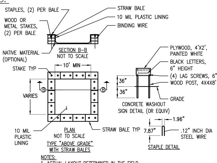
1. ACTUAL LAYOUT DETERMINED IN THE FIELD. 2. THE CONCRETE WASHOUT SIGN SHALL BE INSTALLED WITHIN 32' OF THE TEMPORARY CONCRETE WASHOUT FACILITY.
