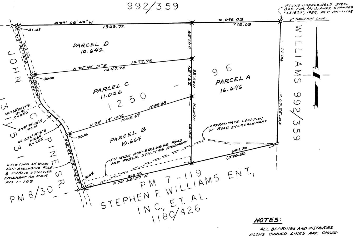
ALL BEARINGS AND DISTANCES ALONG CURVED LINES ARE CHORD MEASUREMENTS.
