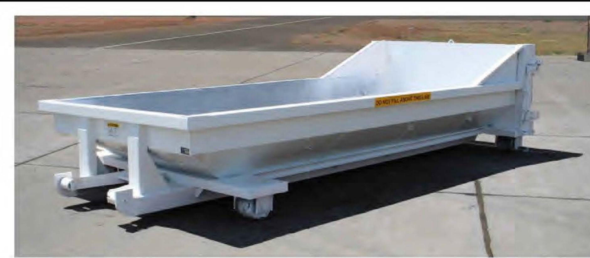
ER-1 PORTABLE CONCRETE WASHOUT CONTAINER NO SCALE
